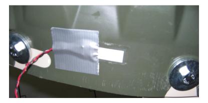
We recommend using duct tape to support the wires. This will prevent the sensor from flexing and increase its life. The wires go under the two center screws.
