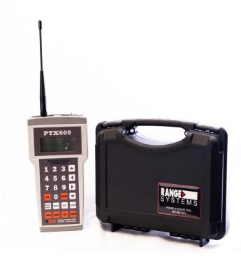
The target controller for Range Systems' Pro Series (Pro-Sniper, Pro-Sniper HD, Pro-SIT) of programmable, portable, pop-up, shoot/don't shoot, and reactive steel sniper target systems now features USB connectivity, back-lighting, and a range of up to 600 meters.
